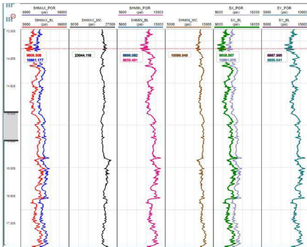
**Figure 6c.** Comparing the results of few of the methods for estimating horizontal stresses on GeoFit™ geomechanics module
