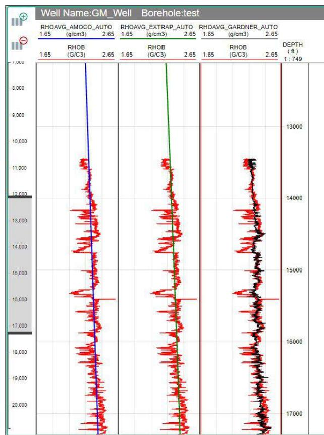
**Figure 6a.** Overburden stress predictions on GeoFit™ geomechanics module
