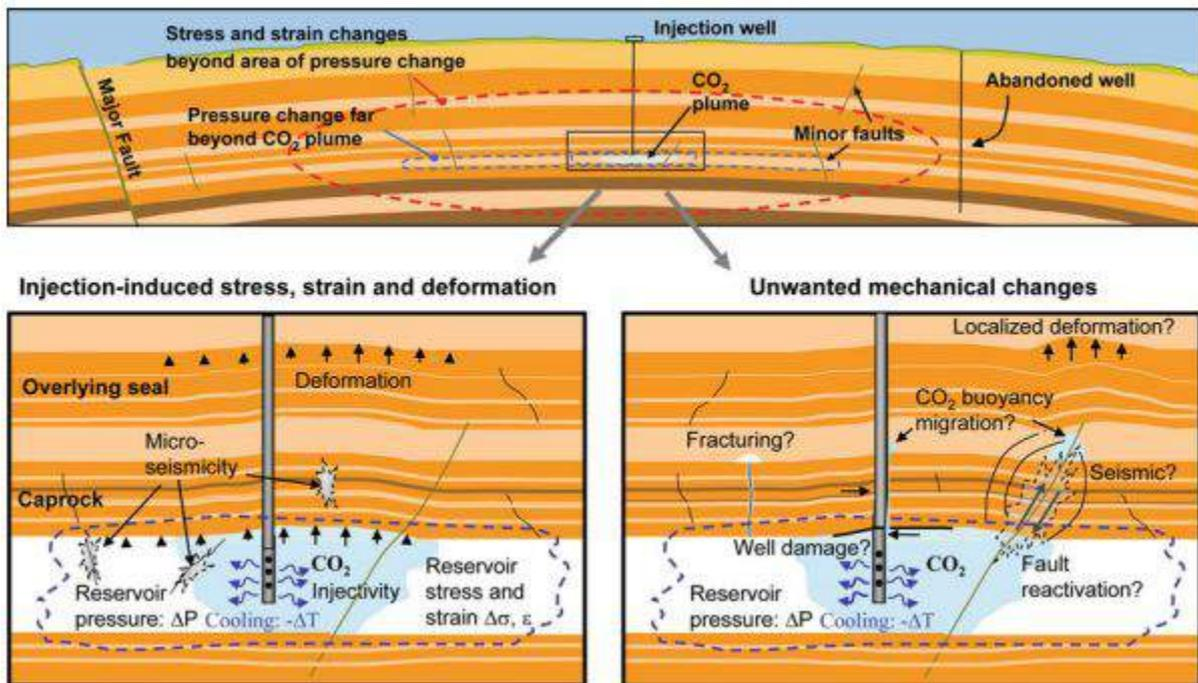
**Figure 2.** Geomechanical processes associated with GCS in sedimentary formations. Pressure and temperature changes induce stresses and strains in the reservoir and cap rocks, thus increasing the chances for fault activations and reduction in sealing capability. (Rutqvist 2012)
