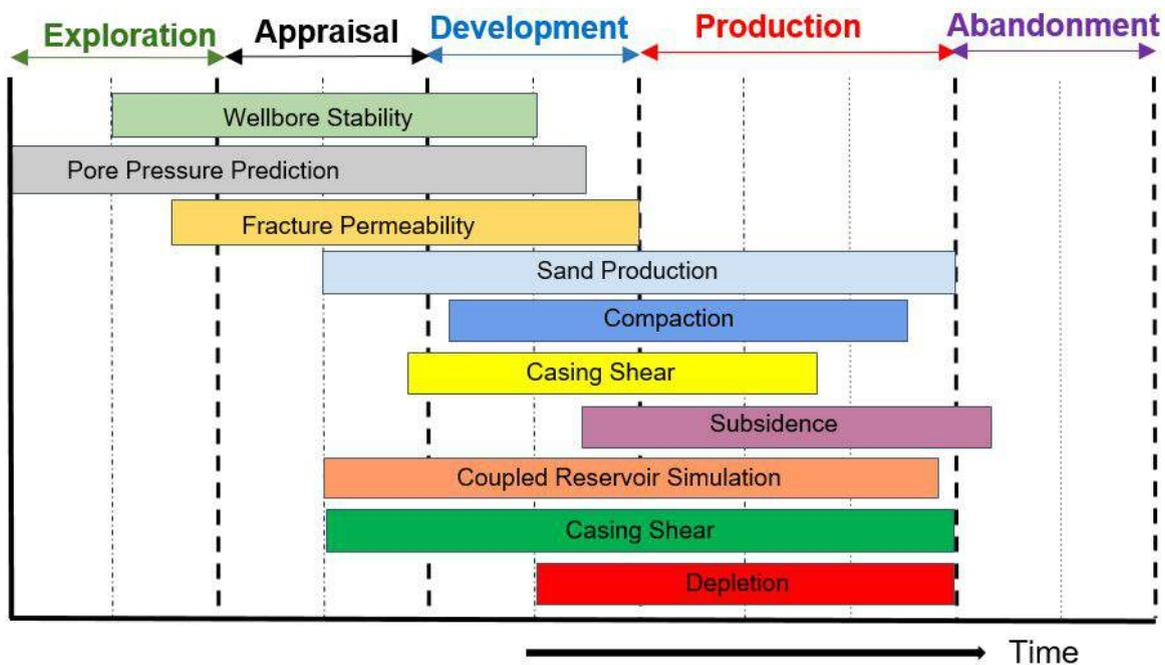
**Figure 1.** Geomechanical applications at different phases of asset development in the oil and gas industry.
