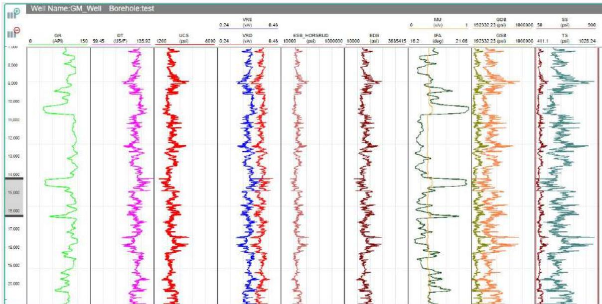
**Figure 6b.** Elastic properties of an Isotropic Rock on GeoFit™ geomechanics module
