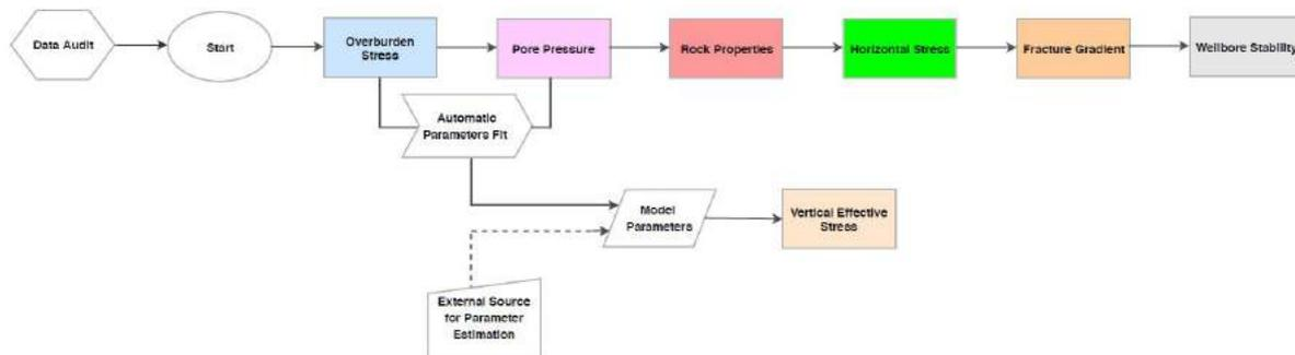
**Figure 5.** GeoFit geomechanics workflow
