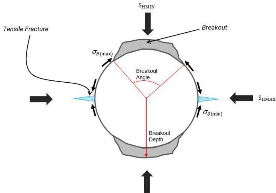
**Figure 4.** Tensile and compressive shear failure around vertical well.
