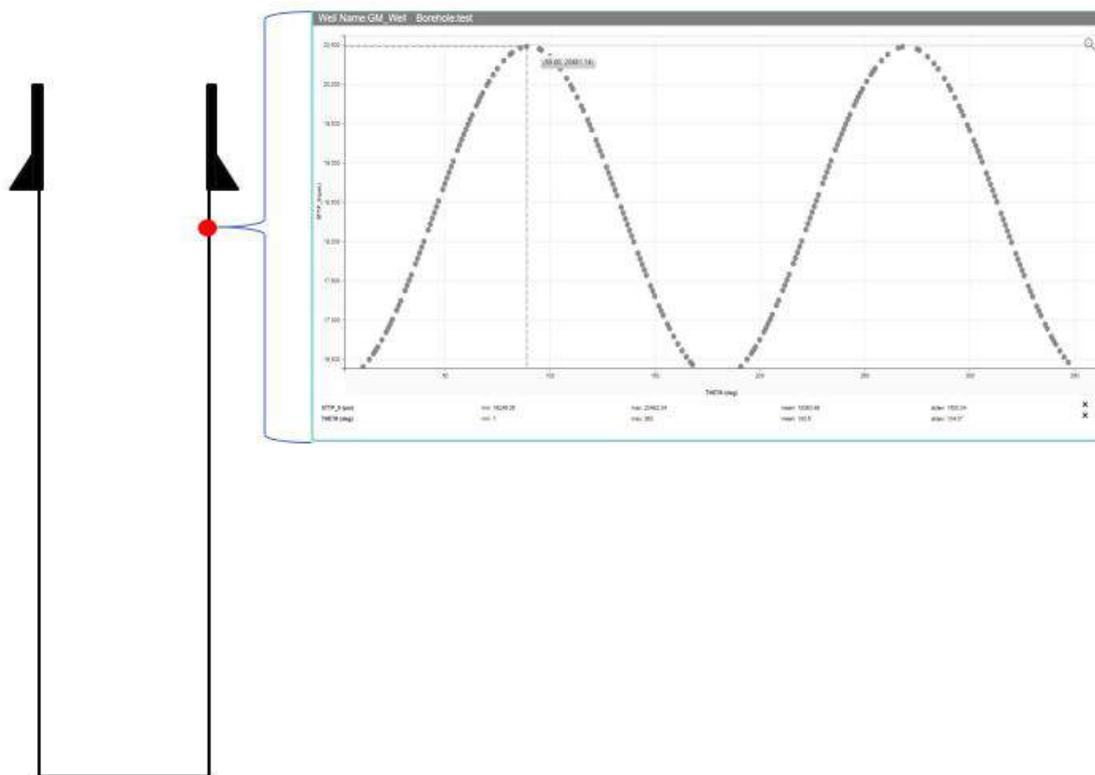
**Figure 8.** Single-Depth Sensitivity Analysis estimates the variation of variable of interest around the wellbore orientation angle.
